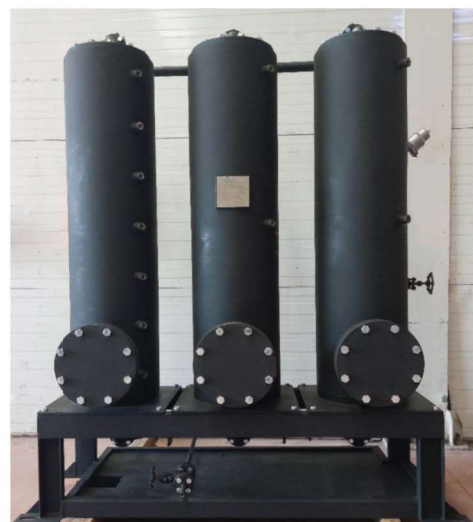
Column Module (Bank) for Mobile Oil Regeneration Plant
