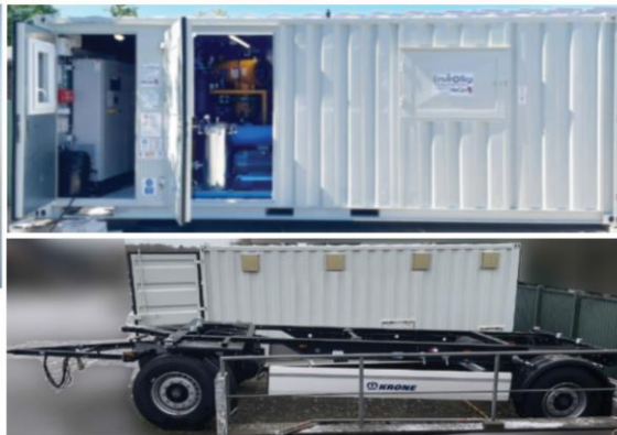
ReGenX-2000, Mobile in 20-foot Container, 6 Columns - 2000 l/h
