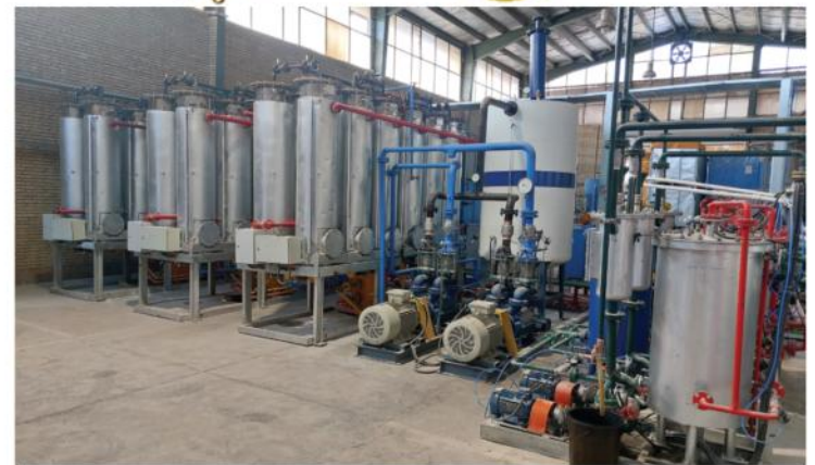
POLISHLUBE PLANT, 3 Bank, 36 Jacketed Reactors, Contains 6500 kg TURBOSORB Adsorbent, 15 ton/day
