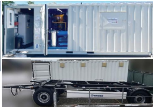
ReGenX-2000, Mobile in 20-foot Container, 6 Columns - 2000 l/h
